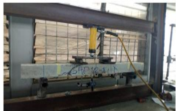
Plate 3.9 Beam Failure for Flexural Test
